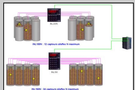
The INL150N is an monitoring unit allowing combination of a large number of temperature sensors in a single device. The « all digital » technology of the whole, reduce significantly the wiring and implementation costs, the sensors being interconnected on a 3 wires bus.
