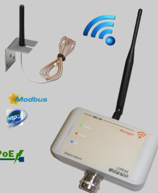
The SML160 is a wireless receiver with an Ethernet connection, the product centralizes all measures issued by the radio transmitters, and makes them available through a standard communication protocol (Modbus-TCP) on the Ethernet link.
